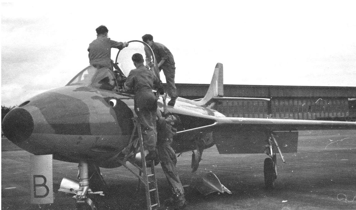
**RAF Bruggen, replacing a canopy. I'm standing in the cockpit**
